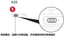
Connect the USB cable to the device and set the switch to the middle position for wired mode
